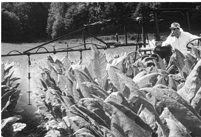
Figure 9-2. Spraying fungicides in burley tobacco with a high-pressure hydraulic boom sprayer with drop nozzles between rows. The proper sprayer provides maximum spray coverage, which is necessary to control blue mold with foliar-applied fungicides.
